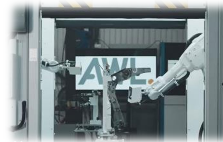
Welding Seam AI Inspection
